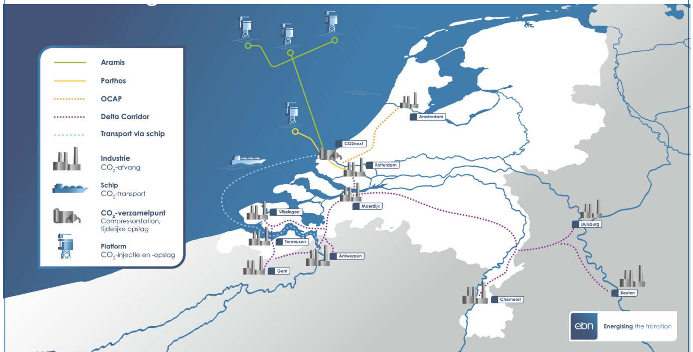
Figure 12: Map of CCS infrastructure in the Netherlands and beyond, including Porthos, Aramis and OCAP
